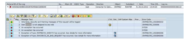
The Application Log shows you the steps processed when the request was executed. Each line represents one step of the request execution. Additionally, you can see a traffic light in front of every line to see where the error occurred. In this case this would be line 3.
